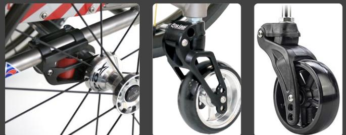
The Hornet has suspension options for the rear wheels (left) - add 500gm
